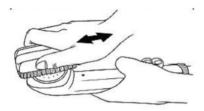
**Is the shower clogged?** Loosen the screw cover and the star squad. Put the strainer in vinegar for a couple of minutes up to an hour. Then reassemble and gently brush the strainer while letting the water flow. Also make sure that the air inlet is open.
